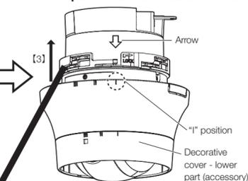
[4] Push the decorative cover up until it is approx. 10 mm {13/32 inches} from the ceiling, and then turn the decorative cover by approx. 16° in the direction of the arrow (clockwise as seen from the bottom) of the figure below.
