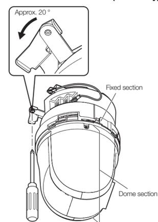
[4] Rotate the fixed section by approx. 20° counterclockwise to detach the camera from the camera mount bracket.
