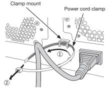
①Pass the power cord clamp through the clamp mount.②Make a ring with the power cord clamp as shown in the illustration to tighten the power cord.
