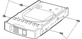
HDD fixing screws for the HDD canister
