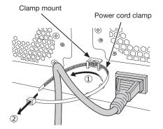
①Pass the power cord clamp through the clamp mount.
