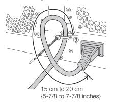
(3)Tighten the power cord at 15 cm to 20 cm {5-7/8 to 7-7/8 inches} from the connector and fix it to the clamp mount.
