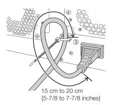
③Tighten the power cord at 15 cm to 20 cm {5-7/8 to 7-7/8 inches} from the connector and fix it to the clamp mount. Cut the unnecessary part of the power cord clamp as necessary.
