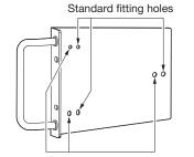
Fitting holes for the front position (about 15 mm {19/32 inches})
