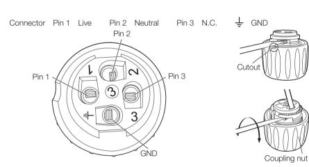
(6) Insert and fix the internal strain relief on the connector as shown in the illustration. Next, rotate the screw of the internal strain relief, and fix the power cord firmly with the fixing
