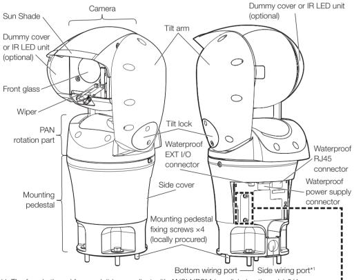
\*1 The female thread for conduit is compliant with ANSI NPSM (parallel pipe threads) 3/4 or ISO 228-1 (parallel pipe threads) G3/4.
