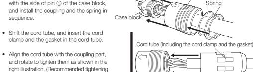
Mount the coupling and the spring on the case block, and tighten the cord tube with the gasket
